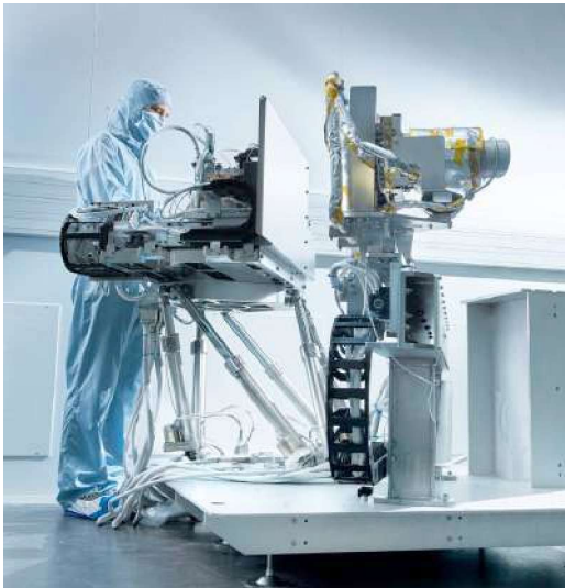
ISO5 clean room compatible hexapod to test space optical instruments for MTG (Meteosat Third Generation) satellites at BERTIN Technologies.
