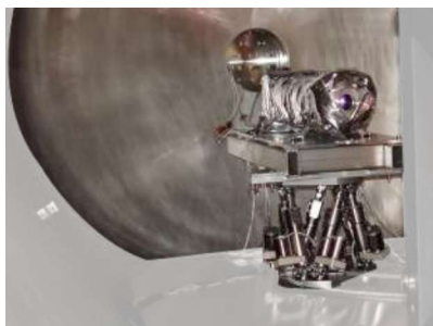
This ZONDA S positions a coronagraph in order to characterize it in a vacuum chamber at Liege Space Center (CSL).
